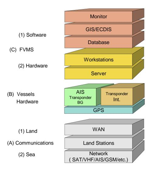
All pelagic longline vessels (currently about 40) are required to carry and operate the shipboard VMS units (sometimes called "transponders") as a condition of obtaining a permit to fish in inland or outside Black Sea waters.
